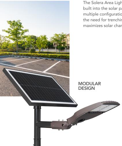
The Solera Area Light features a modular design. The battery is built into the solar panel, and the light engine can be mounted in multiple configurations. No need for a power source, which eliminates the need for trenching & wiring. High performance solar controller maximizes solar charge under all conditions.
